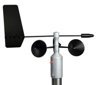
Combined wind speed and wind direction sensor. This sensor range includes, in a single apparatus, transducers for both wind speed and wind direction measurement. Its use simplifies installation requirements, other than being smaller, lighter and cheaper than the general 2-sensors kit. Accuracy and thresholds are anyway near to be comparable with a 2-sensors cup and vane kit alternatives. Different data output signals are available.
