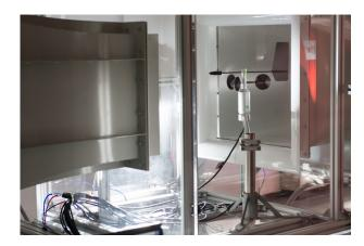
▶ LSI LASTEM is an ISO17025 accreditaded laboratory for air speed measurements. All sensors manufactured are tested inside this laboratory. LSI LASTEM provides Test report for any sensor supplied and on request, ISO17025 or ISO9001 calibration certificates (see Accessories list).
