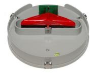
▶ The LSI LASTEM's rain gauges has been developed taking the Class A standard as a reference. (UNI11452-2012 Hydrometry - Intensity of liquid precipitation on the ground - Metrological requirements and test methods for rain gauges). The Class A assures an accuracy over intensity of 3% within 0÷300 mm/hr range.
